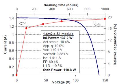
Figure 3: I(V) characteristic and parameters of a 1.4 m<sup>2</sup> a-Si:H single junction module comprising the absorber3 layer with a thickness of 220 nm. On the secondary axis the relative light induced degradation of corresponding cells is shown. A stabilized module power of 110.8 W is achieved.
