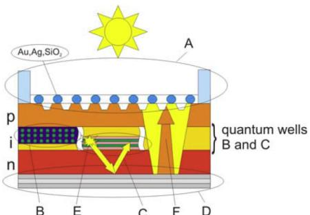
Fig. 1. An idea of proposed solar cell structure,
