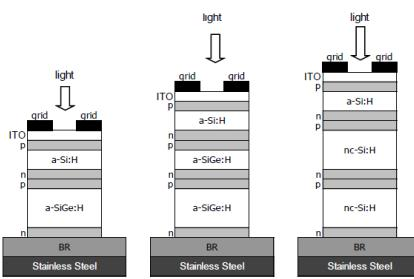
**Figure 1:** Schematic of three a-SiGe:H and nc-Si:H based multi-junction cell structures investigated in this study.
