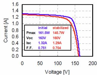
Figure 5: Characteristic of a-Si/mc-Si tandem junction module
