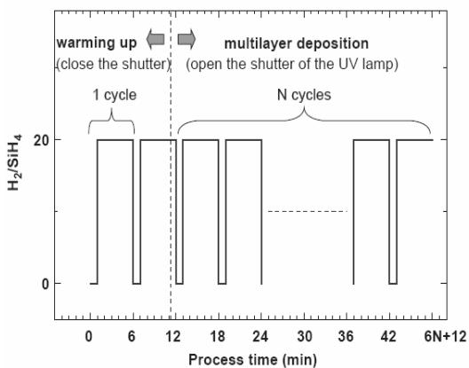
Schematic diagram of alternated hydrogen dilution for an i-pc-Si:H multilayer deposition
