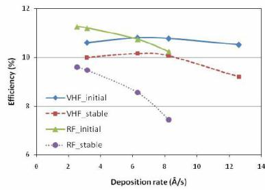
**Figure 2:** Initial and stable a-Si:H/a-SiGe:H double-junction cell efficiency as a function of a-SiGe:H layer deposition rate. The active-area cell size is  $0.25\text{ cm}^2$ .
