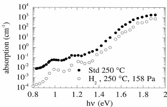
Fig. 3. CPM spectra of a ‘standard’ sample and of the best sample of the  $\text{H}_2$  series.
