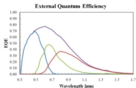
Fig. 4 : EQE of an triple cell with IR of a-Si:H/μc-Si:H/μc-Ge:H solar cell simulated with Sentaurus TCAD. The purple line describes the EQE of the whole cell, the blue, green and red curves the EQE's of the top (180 nm), middle (3 μm) and bottom (90 nm) cell.
