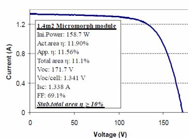
Figure 6: I(V) curve and parameters of a typical Micromorph module that includes the latest processes developed in the Oerlikon Solar pilot line. The low relative degradation due to the new top cell allows for stabilized total area efficiency over 10%.
