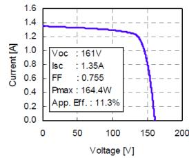
Figure 8: Initial characteristics of a-Si/mc-Si tandem module with increased thickness of absorbers.
