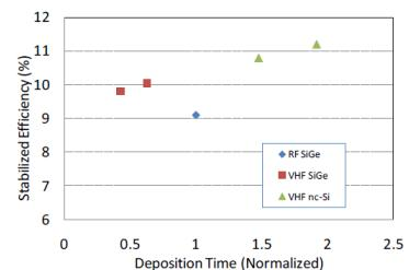
**Figure 5:** Best stabilized efficiency of large-area encapsulated cell, with aperture area of ~400 cm<sup>2</sup>, as a function of deposition time, normalized to the current RF manufacturing time at USO.
